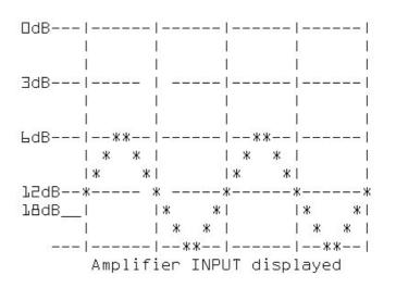
IF YOU WANT TO DO IT MATHEMATICALLY ... Vout = 4Vpp Vin = 1Vpp Therefore, voltage gain Av = Vout/Vin = 4v/1v = 4and gain in dB is: dB =  $20\log(Av) = 20\log(4) = 20(0.602) = 12dB.$
