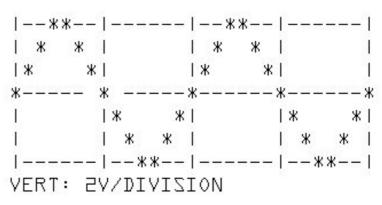
the sidetone oscillator in your QRP rig. Set up the scope for 1v/div, AC volts, and a sweep speed of 1mS/div. Connect the scope probe to the audio output of your rig and set the volume control on key DOWN so the audio sinewave is 2 division peak-to-peak. This would then be 2Vpp AC, and should look similar to the illustration above.
