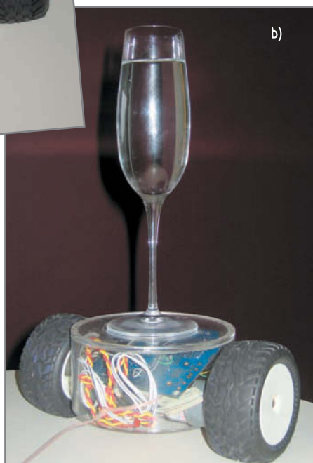
Photo 1a —This is the base of the DanceBot with wheels mounted on motors with quadrature encoders, the logic board powered by the Parallax Propeller, and the miniature camera with an ADC module. b —This autonomous balancing robot uses vision to interact with users. Here it's getting ready to balance a champagne flute for a month.
