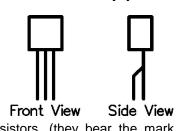
"3904"), as shown in the drawing above. Avoid excessive bending as this can damage the component. Install the reset supervisor into U3, install the PNP transistor into Q3, and install the NPN transistors into Q1, and Q2.
