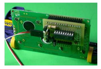
(1) 1x14 or 1x16 (J2), socket header, inserted from bottom of board soldered on top (component) side. Despite the fact that pins 7-10 are usually unused, it is recommended to use a socket (or pin) header with all 14-16 pins as this provides the most rugged mounting rarely requiring anything further to secure the lightweight K107 to the display.
