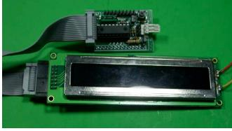
(4) 2x8 (J3) pin header to connect to ribbon cable, inserted on top side, soldered on bottom side. Hold-ing the K107 board with chip writing readable and J3 on the left, J3-1 will be the upper right pin.
