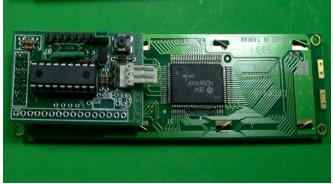
(3) 2x8 (J3) socket or pin header direct to display, inserted on bottom of board, soldered on top side.
