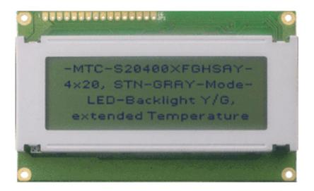
It seems this type display comes pre configured to have its LED backlight always ON. if you plan to use it in this fashion, then ignore this message and don't bother installing any of the backlight control circuitry on the K107 (refer to manual) If on the other hand you do wish to use the backlight under software control, you have to make a minor mod to the back of the display.
